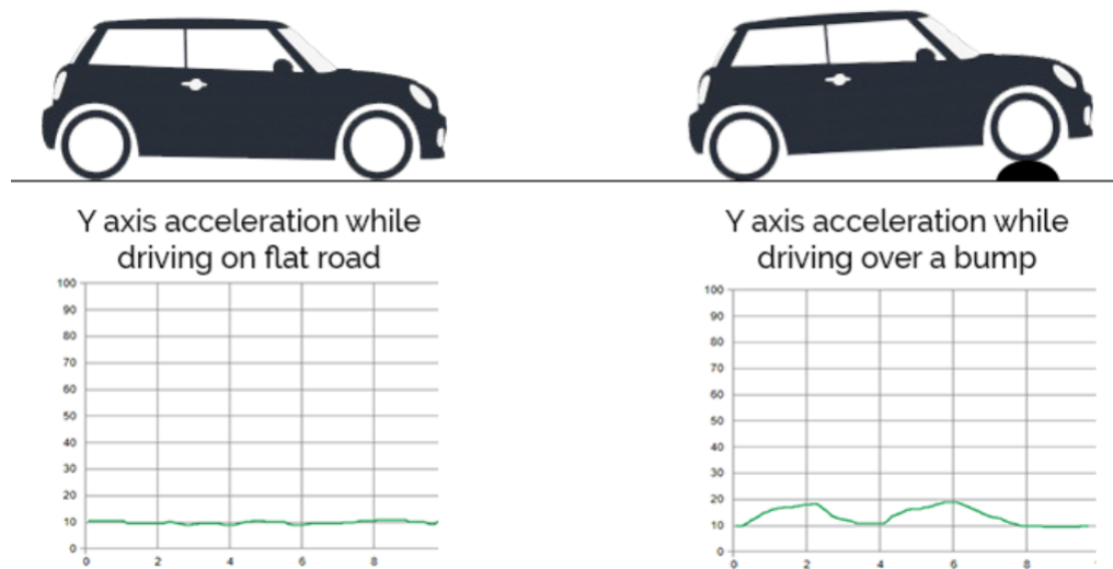
FIGURE 4.6: Bump detection using accelerometer
