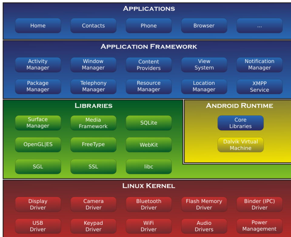
FIGURE 3.2: Android platform architecture
