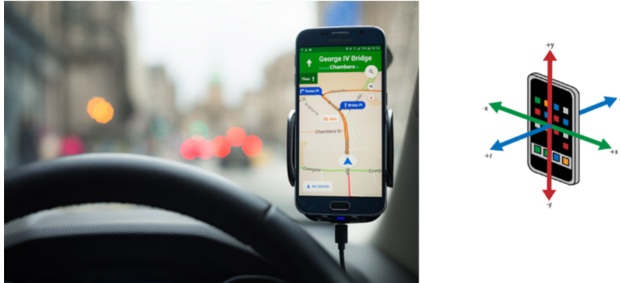
FIGURE 4.5: Smart phone accelerometer axis and the required position when using the application
