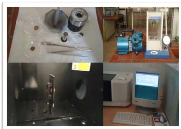
Figure II.5: Instrumentation de la spectroscopie infrarouge (Shimadzu).
