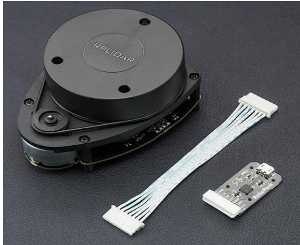
Figure IV.11 RPLIDAR With USB Adapter.
