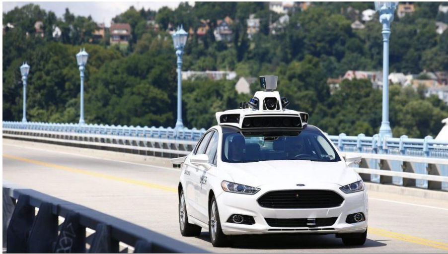
Figure II.17 Self Driving Car With LIDAR And Camera.
