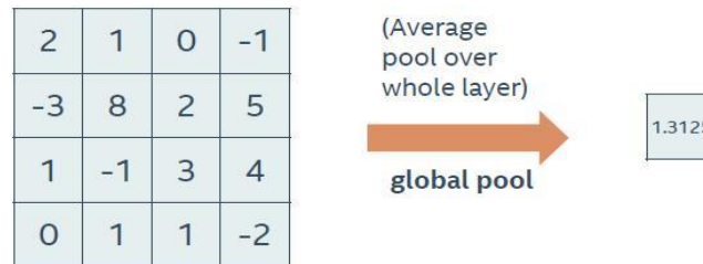
Figure 2.17 - Exemple du global pooling. [17]
