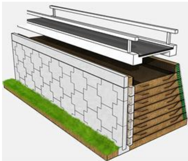
Figure 1.1 Reinforced Soil Retaining Wall.
