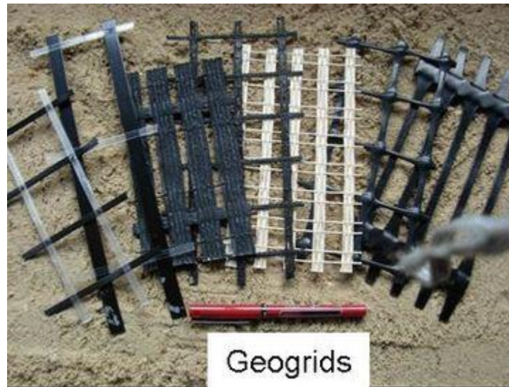
Figure 1.15 Type of reinforcement geogrids.
