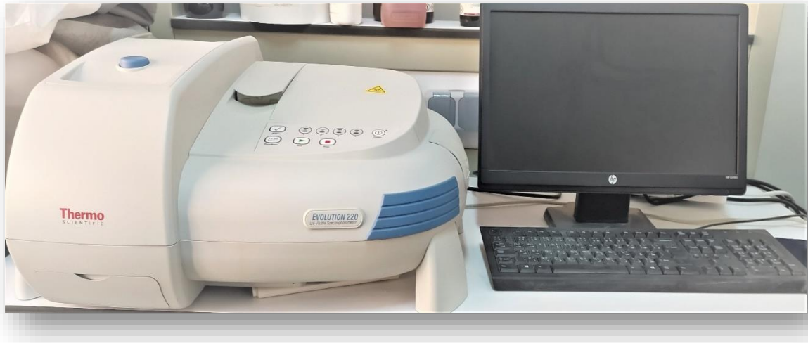
Figure II.10: EVOLUTION 220 spectrophotometer image.
