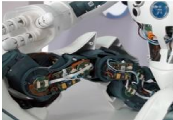
Figure II-4 motors in nao leg [20]
