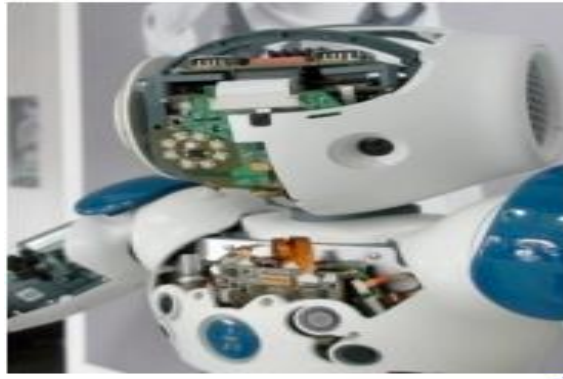
Figure II-1 nao head from inside [20]
