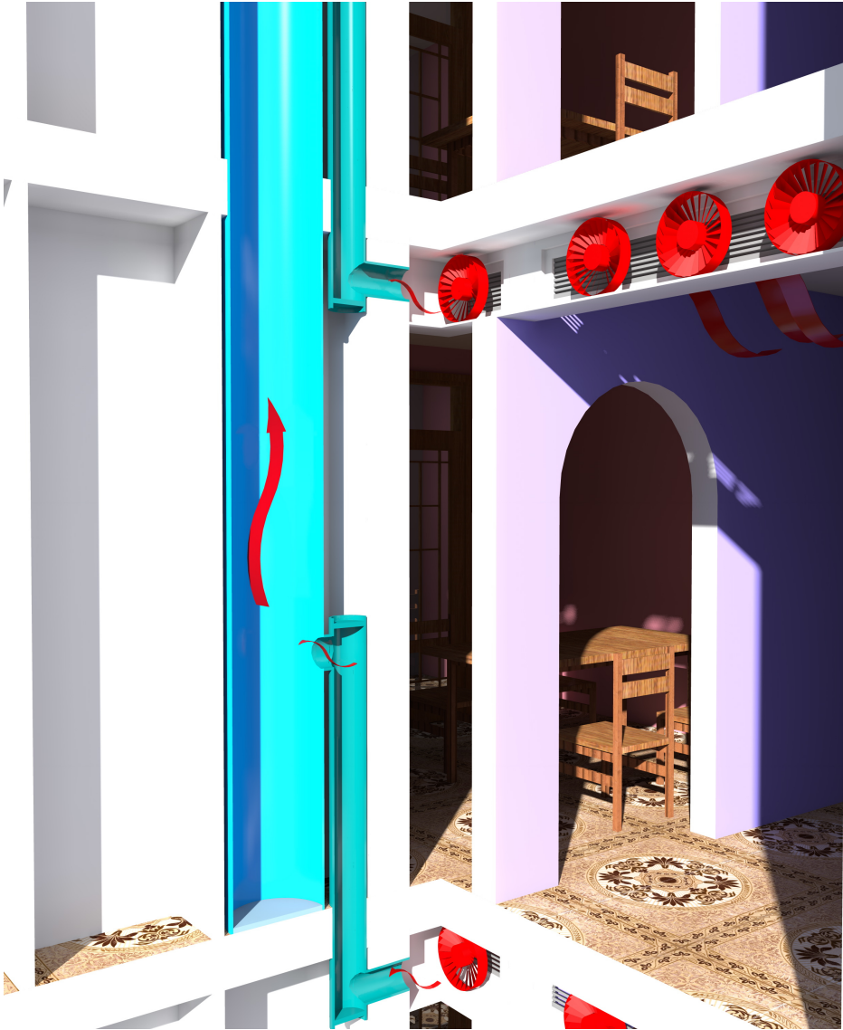
Figure 5.35: Connections to the heat core
