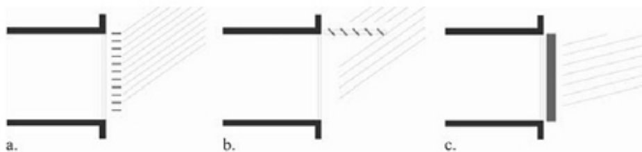
Figure 4.18: Simplified version of current shade devices. (a & b) horizontal shade devices for high angles of radiation. (c) Vertical shade devices for low angles of radiation (morning and evening) [Badarnah 2008]
