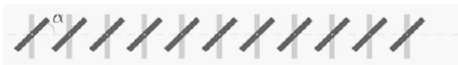
Figure 4.19: All shade blades have the same angle of inclination ( \alpha ) when flipped. Light gray indicates the old position and dark gray the new position [Badarnah 2008]
