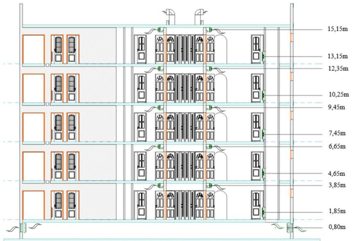
Figure 6.10: Cross section of the new model design representing the different heights for the simulation
