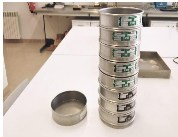
Fig. III.2 Soil sifting equipment
