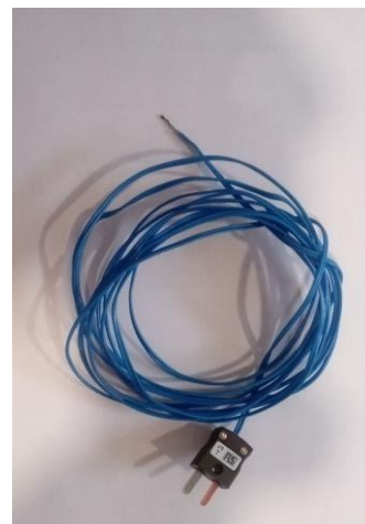
Fig. III.4 Thermocouple type T
