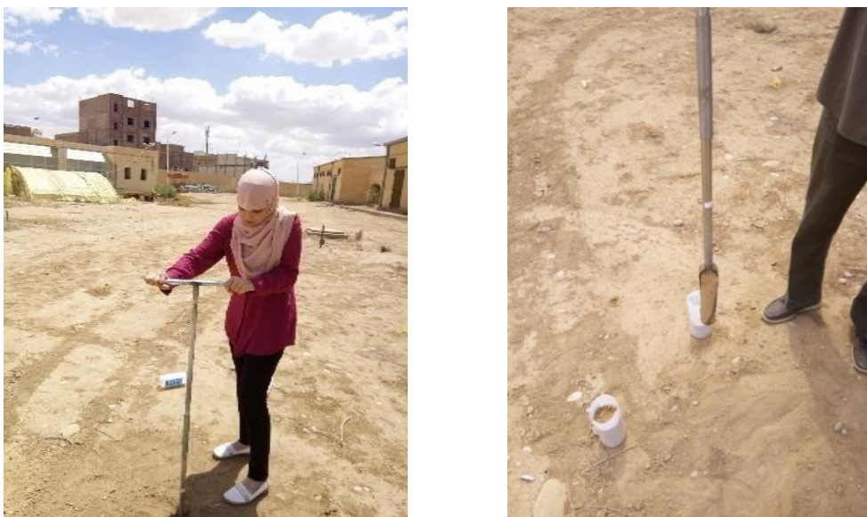
Fig. III.29 Procedure of taking samples with drilling tool.
