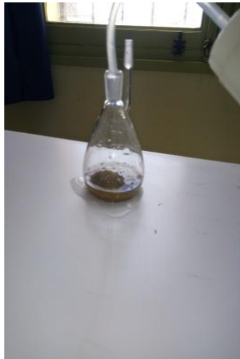
Filling pycnometer by soil sample and distilled water
