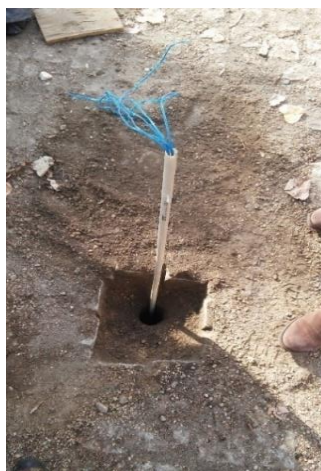
Fig. III.5 Probe inserted in perforated hole
