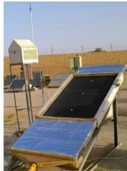
Fig. 5. Photograph of the experimental setup of baffled SAH.
