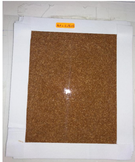
Figure III.15 : Moulage des plaques composites
