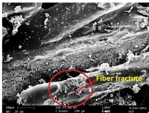
Fig. 11. SEM visualization of C1 sample: Illustration of a fiber fracture.
