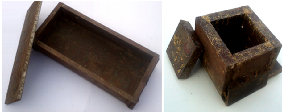
Fig. 3. Metallic molds for three point bending test and thermal conductivity measurements.
