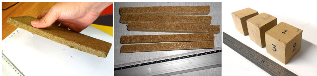
Fig. 4. The plate, specimens and the parallelepipeds composites obtained after compression.
