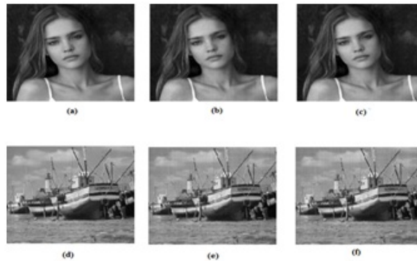
Figure 4.5: Some Examples of Scheme1, (a) and (d) Original Images, (b) Reconstructed Image with 70 SV, (c) Reconstructed Image with 110 SV, (e) Reconstructed Image with 112 SV, (f) Reconstructed Image with 150 SV.
