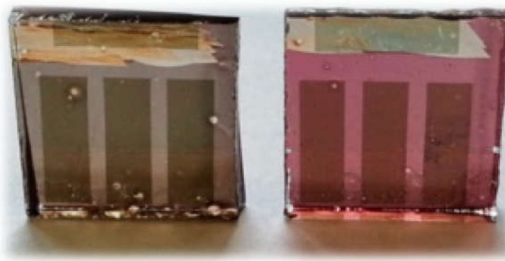
Figure 2. 12: Picture of semitransparent perovskite solar cells without (left) and with (right) D102 dye included in the spiroOMeTAD layer, with 10 nm gold electrodes [55].
