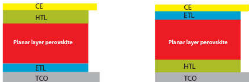
Figure 3. 11: Solar cell structures (n-i-p at left and p-i-n at right).
