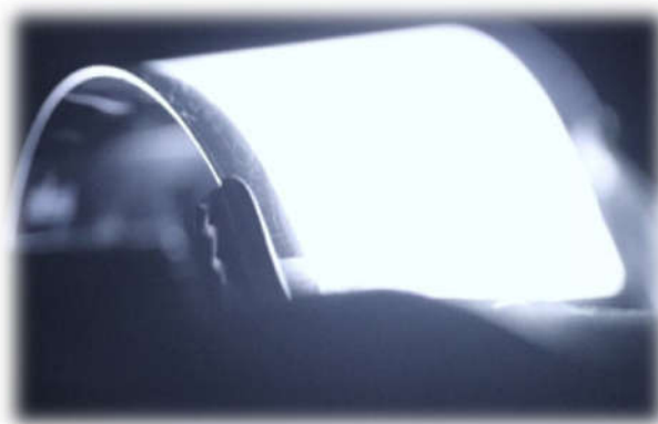
Figure 2. 15: Photograph of near infrared flexible PeLED with large-area [62].
