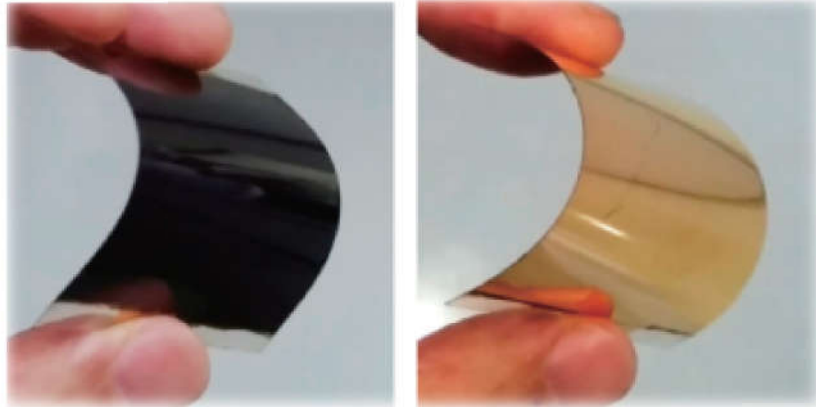
Figure 2. 6: Photograph shows a large plastic film perovskite device (left: perovskite side, right: gold electrode side) fabricated by the low temperature coating methods.
