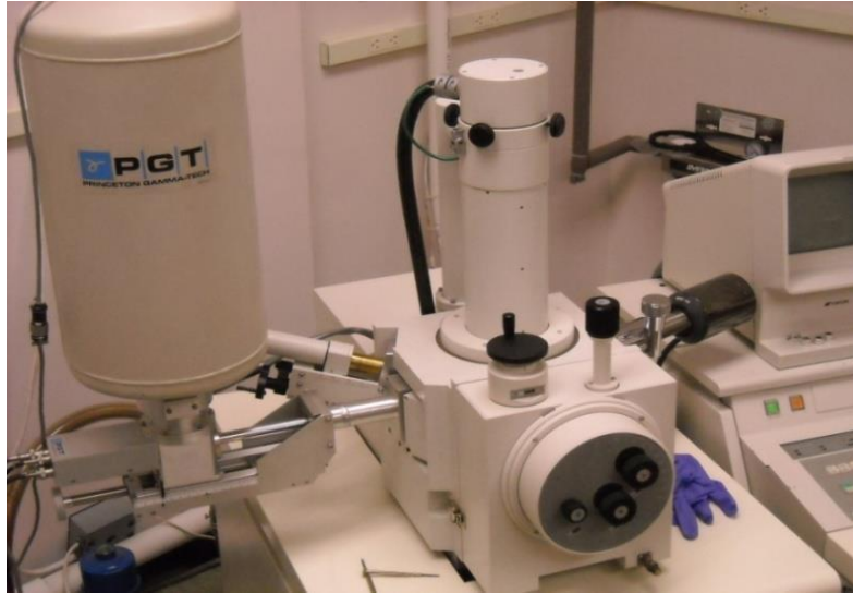
Figure 2.6: Example of energy dispersive X-ray spectroscopy.
