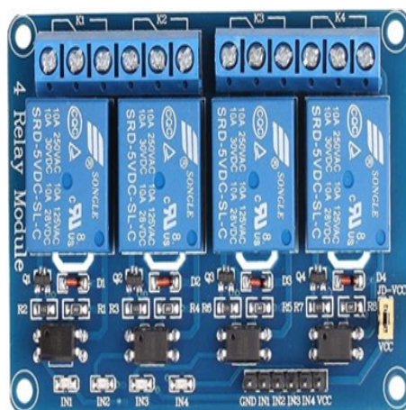
Figure 3.21: Relay module 4 channel
