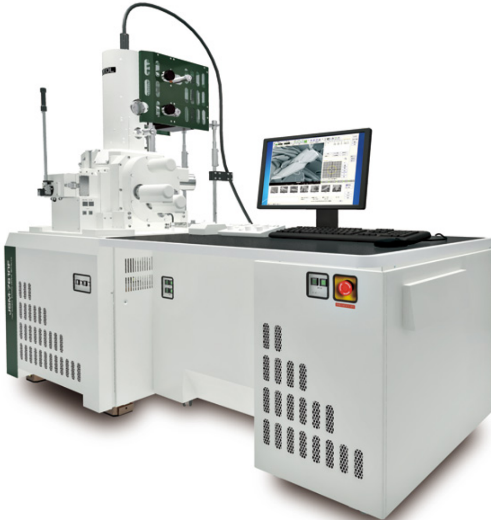
Figure II.6: High-Resolution SEM JSM-7610F Plus (CRTSE, Algeria).
