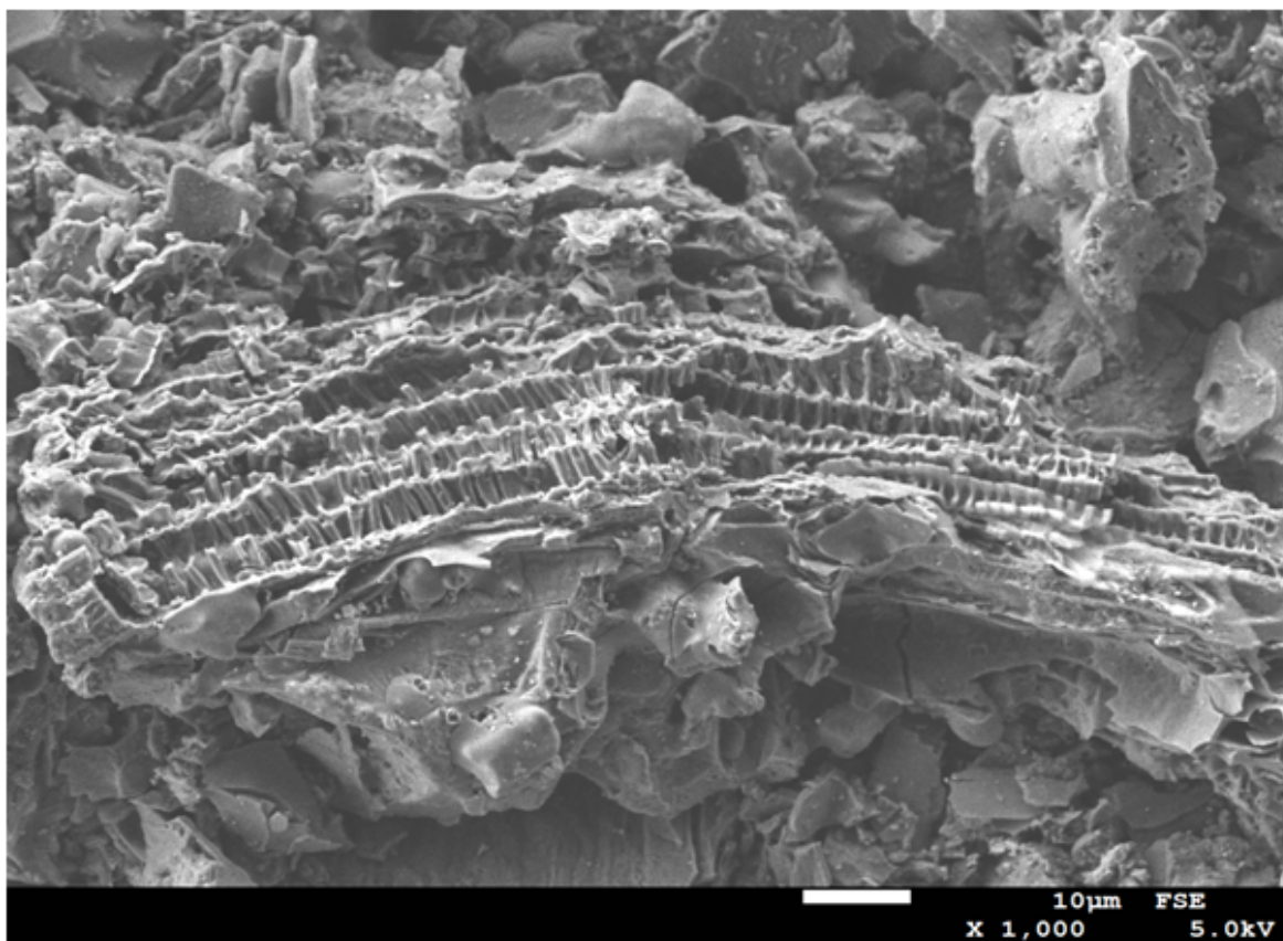
Figure III.5: SEM Micrograph of BC Sample at 10\mu\text{m} , Magnification X1,000.
