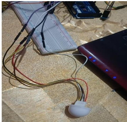
Fig II.18 BH1750FVI assembly real photo
