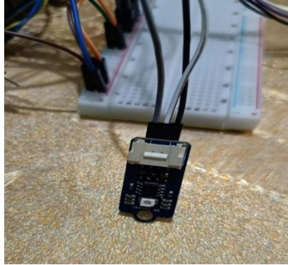
Fig II.24 Assembly of Ultraviolet (UV) sensor in the real photo
