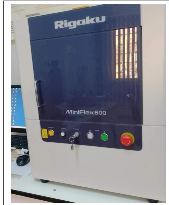
Figure (II .12) : Diffractomètre Rigaku MiniFlex600.
