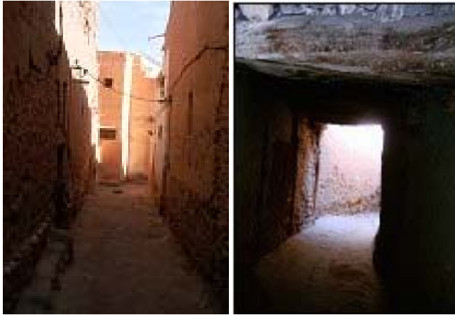
Shape 2: The street offers a mutual shade, the breeze and the preservation of the walls from the sun, and on the other hand it is an important wind breaker. (Source: the author's work out)
